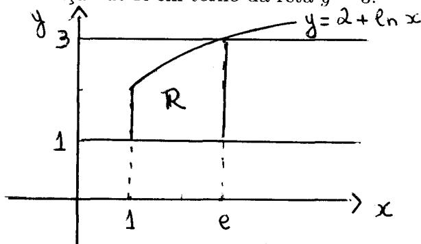
$$\begin{aligned} V &= \pi \int_1^e [(3-1)^2 - (3-2-\ln x)^2] dx = \pi \int_1^e (3 + 2\ln x - \ln^2 x) dx = \\ &= \pi \left[ 3(x-1) + 2 \int_1^e \ln x dx - \int_1^e \ln^2 x dx \right] \end{aligned}$$
